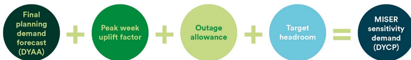
Figure 2 Calculation of MISER demand for DYCP sensitivity analysis
