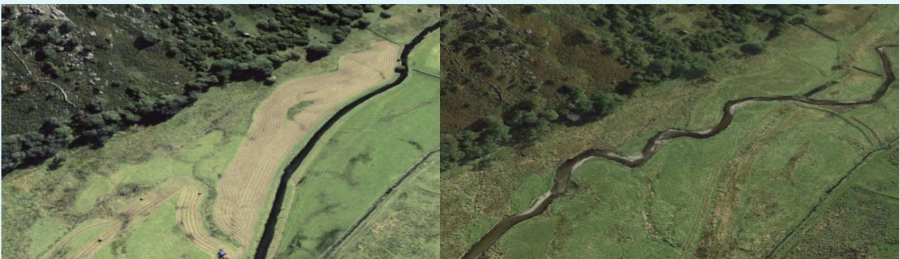
Figure 2-3: The re-meandering of Swindale Beck (shown before, on the left, and after, on the right)
