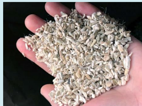
Figure 22: Image of the plant-based media (kenaf) used for MOB
